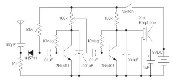
The above schematic shows a 100k volume control but the signals usually aren't loud so this component may
